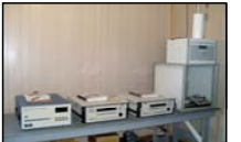
Figure 4: Monitoring equipment (l-r): Ozone (TEI-49C), NO x (Teledyne-API), H 2 S/SO 2 (Teledyne-API), PM 2.5 (MetOne-BAM), FRM – Partisol located outside. The CO 2 , CO and NH 3 monitors are not shown. (Green Horse Society)
